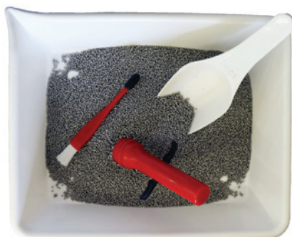
Four simple tools to tame granules: Lipped Tray, Scoop, On-Off Magnet and Brush.
