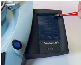
3. Select desired foil (in the example Erkoloc-pro)
