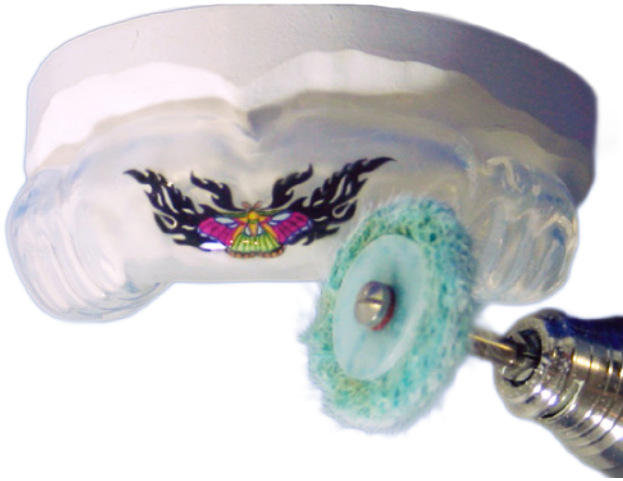
Figure 5. Allow the mouthguard to cool to room temperature then using the Lisko-s disc (art # 223200) lightly smooth the edges into the mouthguard working outwards away from the graphic.
